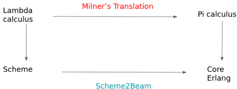
Figure 1: Diagram of translations from \lambda -calculus to \pi -calculus, from Scheme to Erlang, and where our project fits in.
